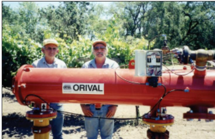
Orival Model ORI-04-PE, equipped with 9V battery controller, protects the Blasi's drip system.
