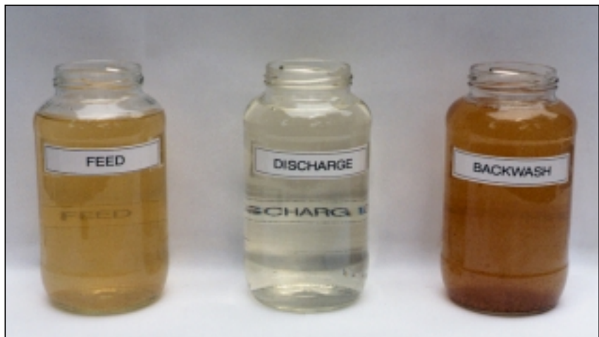
Samples of inlet, outlet and backwash water. Notice the dramatic difference in concentration between the inlet and outlet samples.
