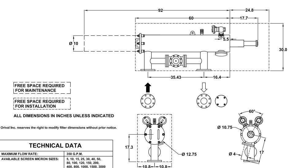
**OPEN AREA STANDARD SCREEN:** 474 SQ. INCHES **OPEN AREA HIGH PERFORMANCE** SINTERED MULTI-LAYERED SCREEN: 713 SQ. INCHES **150 PSIG** MAXIMUM WORKING PRESSURE: MINIMUM INLET PRESSURE REQUIRED DURING RINSE CYCLE: 30 PSIG MAX. WORKING TEMPERATURE: 150°F **INLET/OUTLET FLANGES:** 4" ANSI 150#
